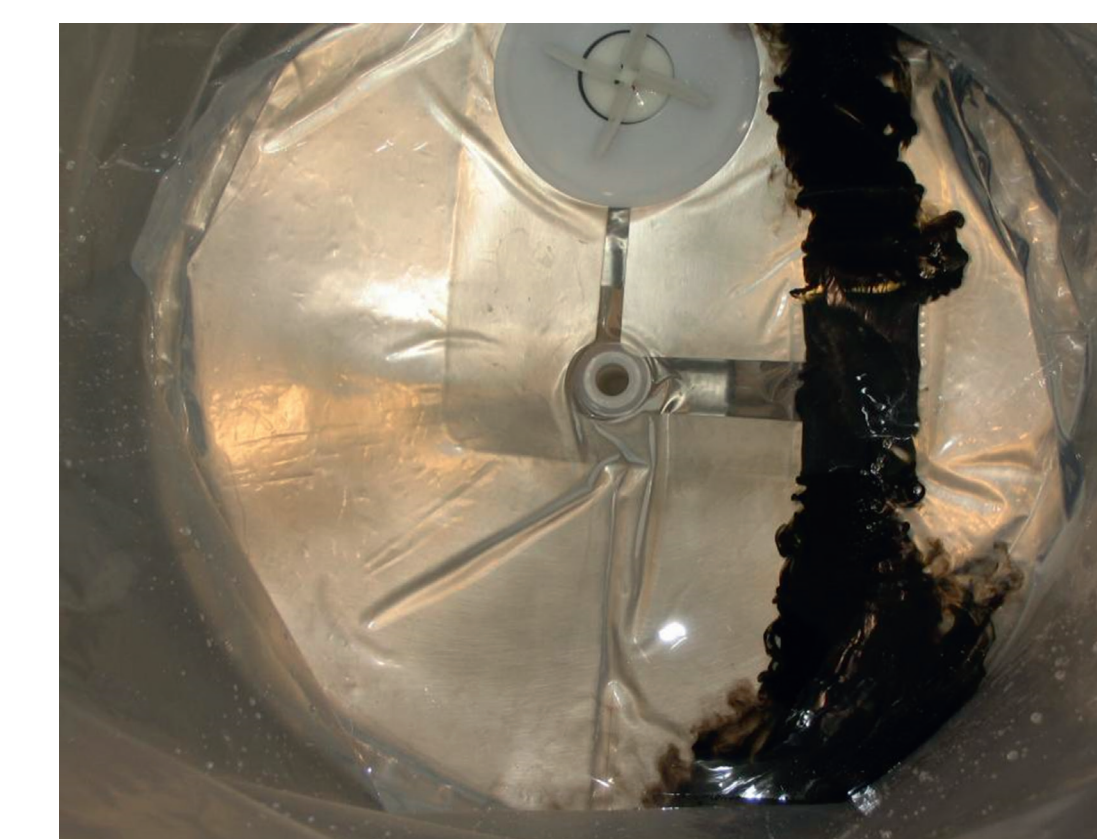
Figure 12: Retentate diverter plate directs return flow tangentially, preventing short-circuiting to the center feed port. Allowing less than 1 L
