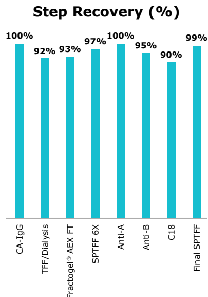
Figure 13. Typical recoveries obtained in the pilot-scale purification.
