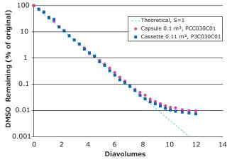
Figure 5. Diafiltration of 20% DMSO from aqueous solution.
