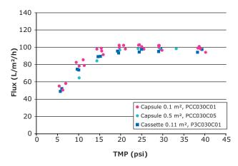
Figure 3. Effect of TMP on permeate flux for Pellicon $^{\circ}$  Capsule and Pellicon $^{\circ}$  cassette; 10g/L BgG.
