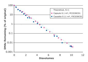
Figure 4. Diafiltration of 20% DMAc from aqueous solution.
