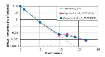
Figure 9. Clearance of 6.8% DMSO by diafiltration of 26-28 g/L ADC mimic.  $^{\rm 6}$
