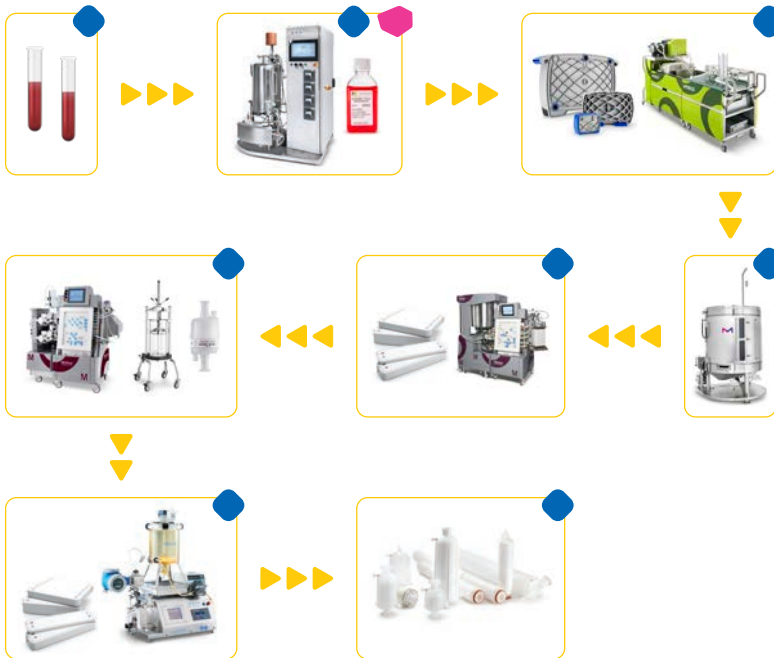
Figure 8. 200L process for adenovirus vector using Mobius® single use systems. The process can be scaled up to 2000L.
