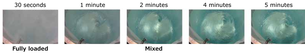
Figure 2. At 2 minutes, process data for mixing 1X PBS in Mobius® Power MIX 2000 shows conductivity reaching final value at both top and bottom of vessel, and particle count reaching minimum. At same time, visual mixing is complete as it is once again possible to see through to the bottom of the vessel. No further changes in measured values or visual were seen after 2 minutes, confirming complete mix at that time.
