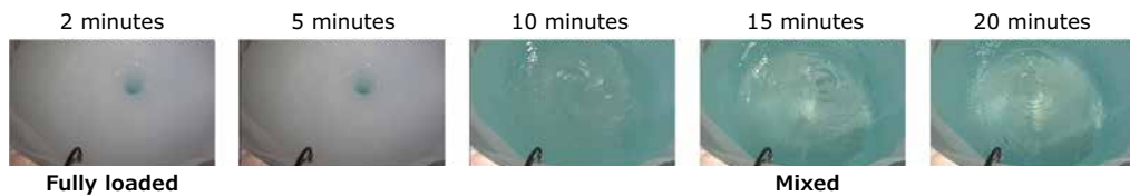
Figure 3. At 5 minutes, conductivity readings at both the top and bottom of the vessel reach a stable value, indicating homogeneity in mixing 1.5M NaCl in the Mobius® Power Mix 2000. However visual mixing is not complete until 15 minutes when it is once again possible to see through to the bottom of the vessel. Particle count reaches a minimum at 15 minutes, where not only distribution, but dissolution is complete. After 15 minutes, there is no change in visual or measured values.
