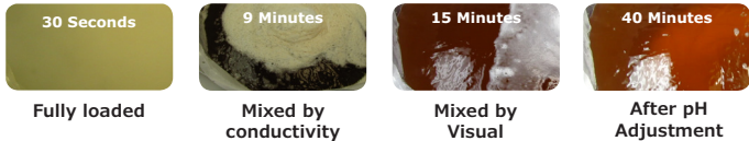
Figure 7. With impeller rpm reduced to 240 rpm, mixing time for Custom medium is increased, but foaming is essentially eliminated. Conductivity reaches a stable value at 9 minutes. The last of the powder is incorporated at 15 minutes for visual mixing complete. At the same time, particle count reaches 99% of the maximum value. After pH adjustment, particle count goes to zero, without any foaming or bubbles.
