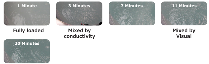
Figure 3. At 3 minutes, conductivity readings at both the top and bottom of the vessel reach a stable value, indicating homogeneity in mixing 1.5M NaCl in the Mobius® Power MIX 1000. Particle count reaches a minimum at 9 minutes. Mixing by visual is deemed complete at 11 minutes, as there is no further change in appearance after 11 minutes.
